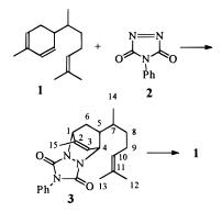
acted zingiberene or excess PTAD were readily removed by chromatography. Thus, after concentration, the mixture was purified by flash chromatography on Si gel to remove the other unreacted hydrocarbons, yielding the pure adduct **3** as a colorless gum. Base hydrolysis of **3**, followed by extraction of the recovered zingiberene into hexanes and Kugelrohr distillation, produced **1** in >99% purity by GC (Scheme 1).
